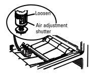
The shutter for the bottom (oven) burner is near the back wall behind the drawer. Remove the drawer. See the *Care and cleaning of the range* section.
